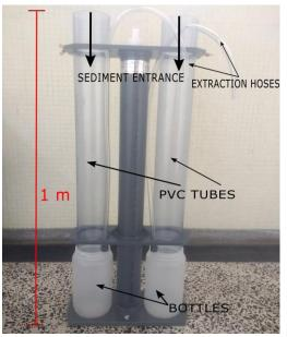
Figure 1 Sediment trap setup.
