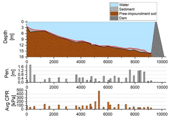
Fig. 4. Longitudinal profile of sediment thickness (top), penetration depth of graviprobe (middle), and hardness (down) in Passauna reservoir
