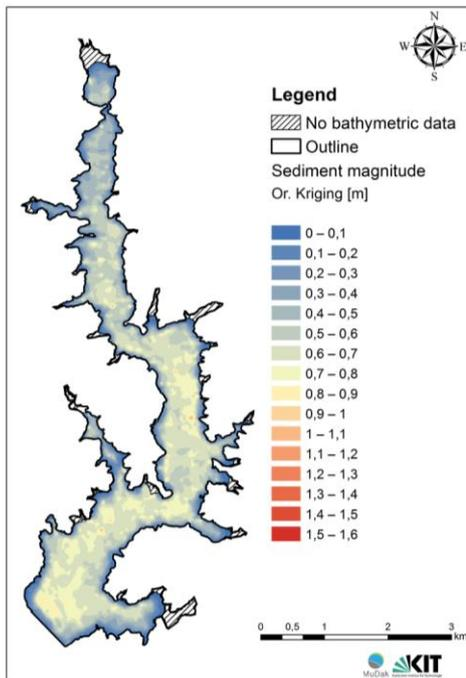
Fig. 3. Spatial distribution of sediment thickness in the reservoir from hydroacoustic measurements
