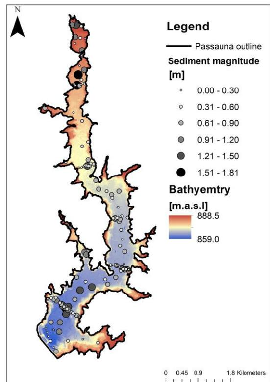
Fig. 2. Locations of GraviProbe measurements with sediment magnitude at the corresponding location, multibeam bathymetry in the background
